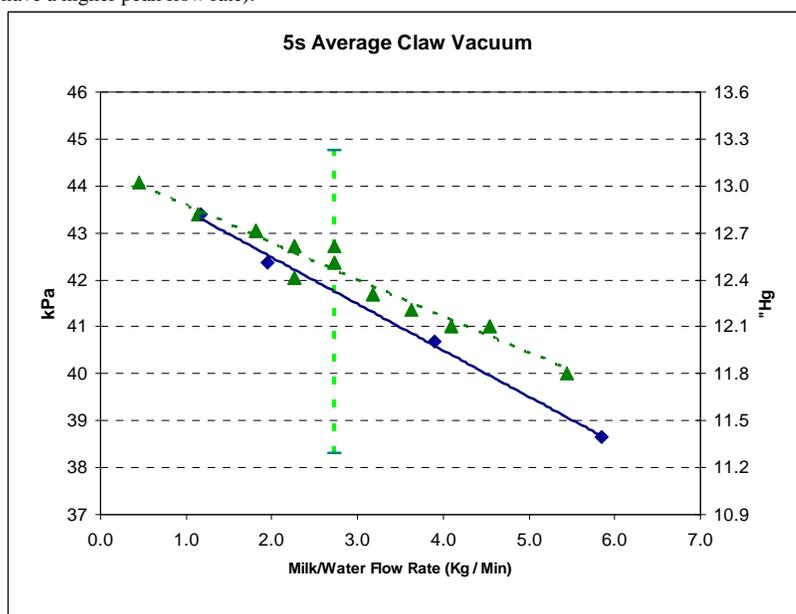
Figure 3. Example Average Claw Vacuum Measurements: wet test, milking-time test without known milk flow rate, and milking-time test with known flow rate.
