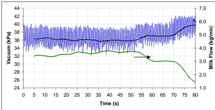
Figure 1. Simultaneous recording of milk flow rate and claw vacuum.
