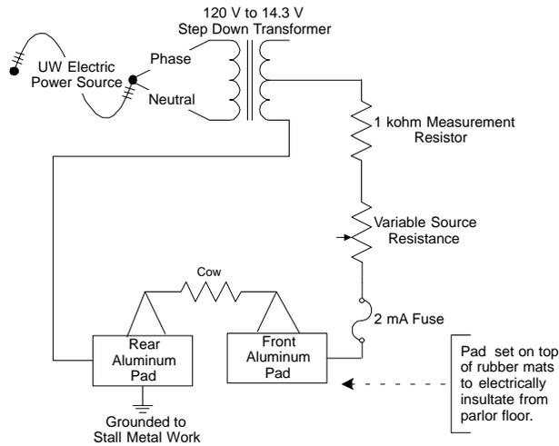
Figure 2. Schematic of electrical apparatus for milking time tests.
