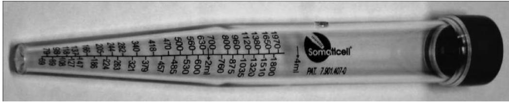
Figure 1. The test vial demonstrating graduation of SCC readings.
